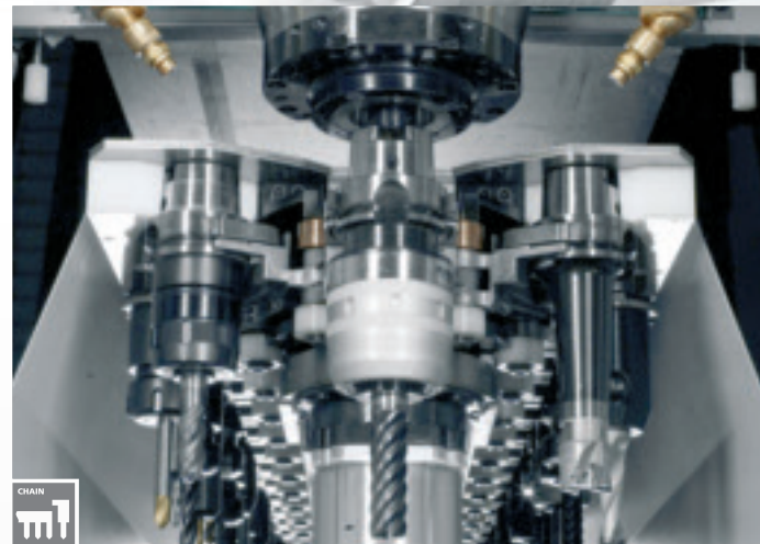
Automatic tool change with the pick-up method as fast as 1.5 s (40 tool places).
